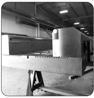
**VEE-LOCK®** Adjustable Dies significant-ly outperform standard shim-style adjustable dies in both productivity and durability. Their unique design allows them to provide a high level of functionality in a wide variety of forming applications. Unlike the shimstyle adjustable dies that require the operator(s) to lift shims in and out of the tool to change the opening, the
