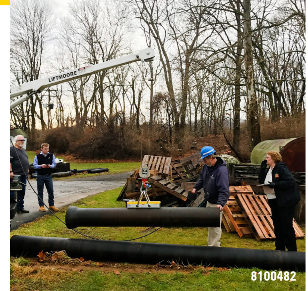
Lifting Pipe with MLAY1000x6 Lifting Magnet
