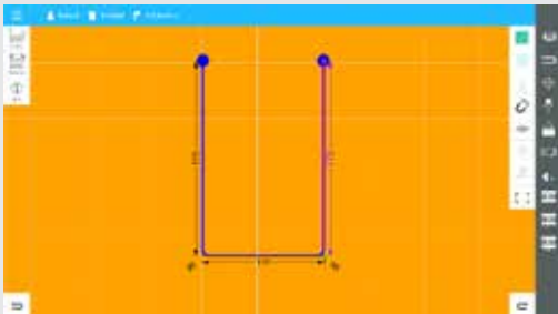
MULTITASKING : workpiece drawing with instantaneous collision detection and calculation of the bending sequence in the background
