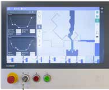
Intuitive Interface with combined numerical-graphical user interface
