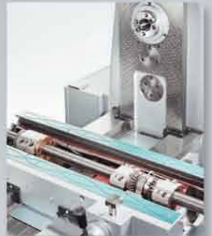
Double box ways on saddle, also showing power feed table driving mechanism.
