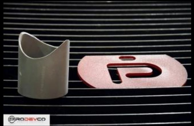
Pipe Cutting using PCR42
