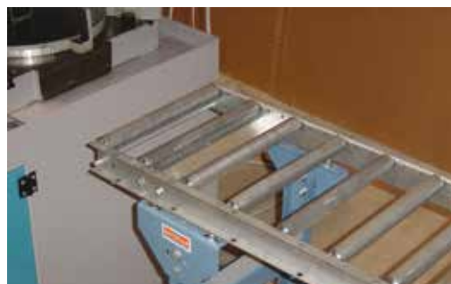
Free standing conveyors available in 5' and 10' sections.
